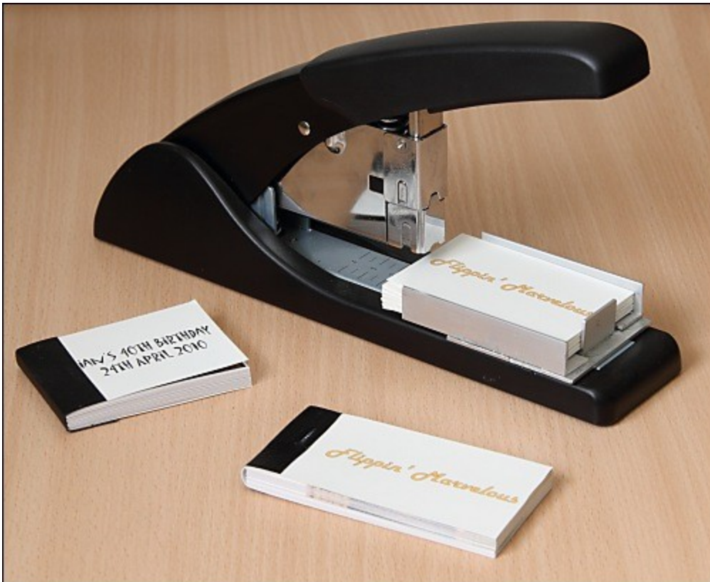
A heavy duty stapler used to bind the books shown here with a jig to hold the pages
