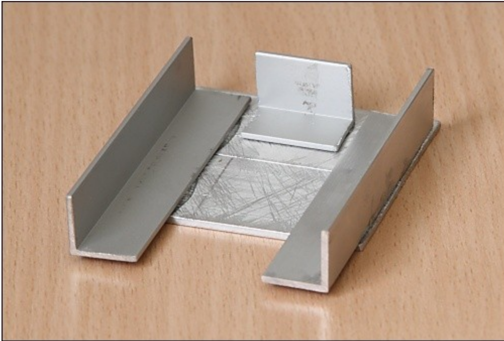
Simple jig for holding the pages for stapling
